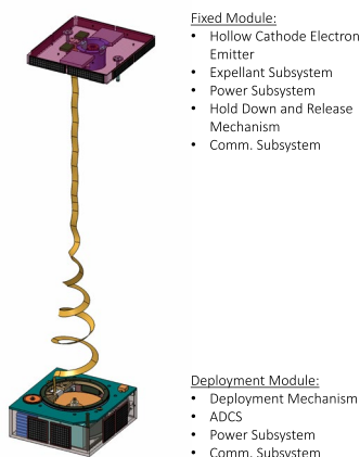
Fig. 2 Basic deployer kit configuration with the interface to the satellite (top), the tape tether and the DM (bottom)
