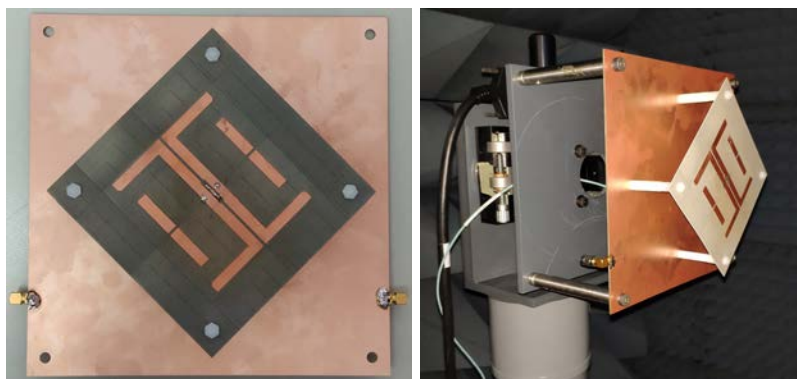
Figure 2.24: Pictures of the antenna prepared to be measured in the anechoic chamber.
