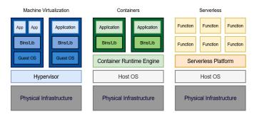
Fig. 1. Differences between the resource models of three cloud paradigms: a) virtual machines; b) microservices; c) Serverless, when developing cloud applications.
