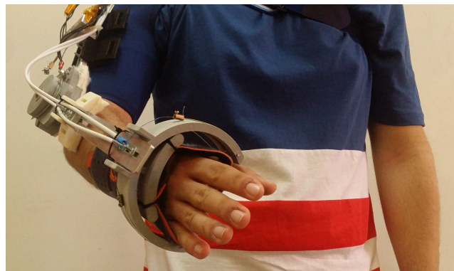
FIGURE 6. Exoskeleton pronation-supination parts. (a) CAD structure for the pronation-supination parts. 1 - actuator termination for Bowden cable, 2 - shaft for pulley, 3 - canal slip, 4 - terminals for traction cable hold, 5 - sliding part, 6 - attachment point (to the hand through a belt), 7 - fixed part, 8 - sliding point. (b) real design.
