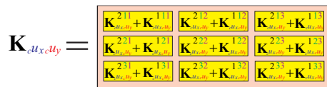
Fig. 14. Finite Element implementation of the Generalized Unified Formulation: example of element matrix \mathbf{K}_{c u_x c u_y} .
