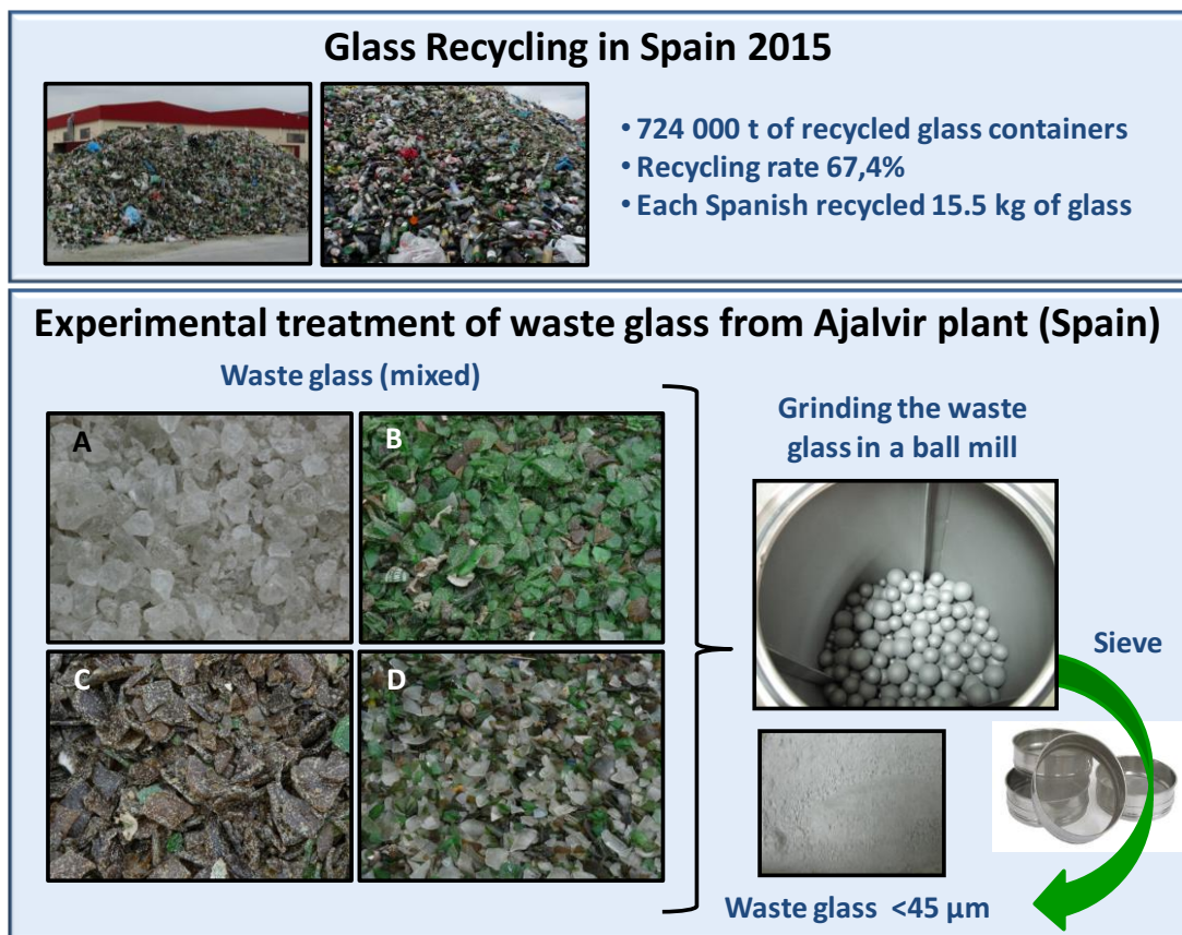
Figure 1. Treatment of waste glass of different colours (from a recycle plant at Ajalvir, Madrid, Spain) to obtain a particle size of < 45 μm for subsequent alkaline activation: A) clear waste glass; B) green waste glass; C) brown waste glass; D) mixed waste glass (used in the study)
