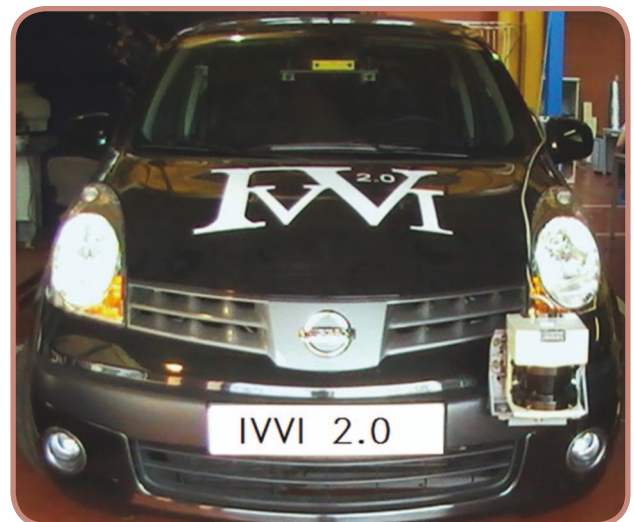
FIG 1 Test platform IVVI 2.0 (Intelligent Vehicle based on Visual Information 2.0) with the sensors visible.
