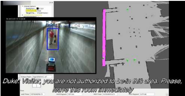
Figure 10: Interactive display showing the restricted zone and a trespassing response with the robot speaking to the intruder.
