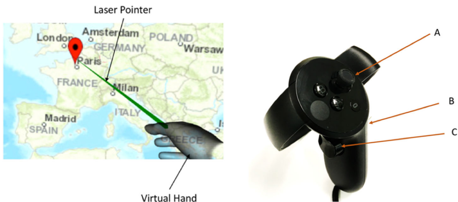
Fig. 2 (Left) Map Interface in Virtual Reality Environments using device-based interaction. (Right) Oculus touch button distribution: A. Thumbstick, B. Index trigger, C. Hand trigger
