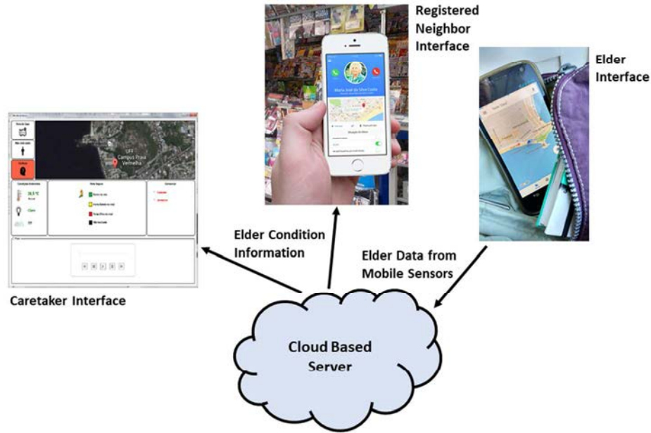
Figure 2: The three different Apps: Relative/Caretaker app, Neighbor app and Elder app (provides sensor data, no interaction needed), interacting with the cloud-based server.
