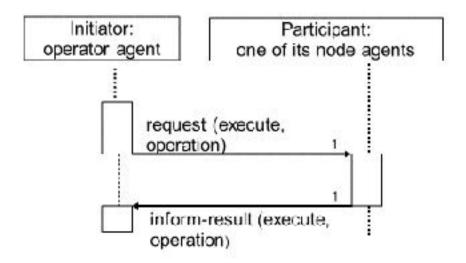
Figure 6: Request plan execution interaction protocol between an operator and a node agent
