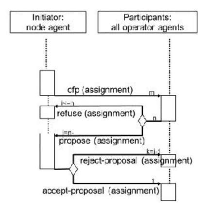
Figure 1: CFP interaction protocol between a node and an operator agent
