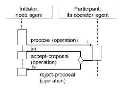
Figure 2: Propose interaction protocol between a node and an operator agent
