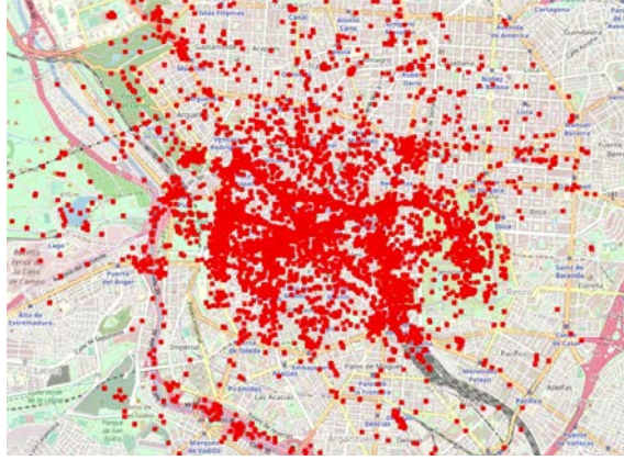
Figure 3.5: Example of a radially decreasing density distribution in the city of Madrid. As we move away from the city center ( density centroid ) the density of samples decreases.
