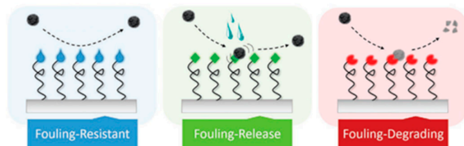
Figure 2. Illustration of the main antifouling strategies, as described by Kamperman et al. (Figure reproduced with permission from Reference [19]).
