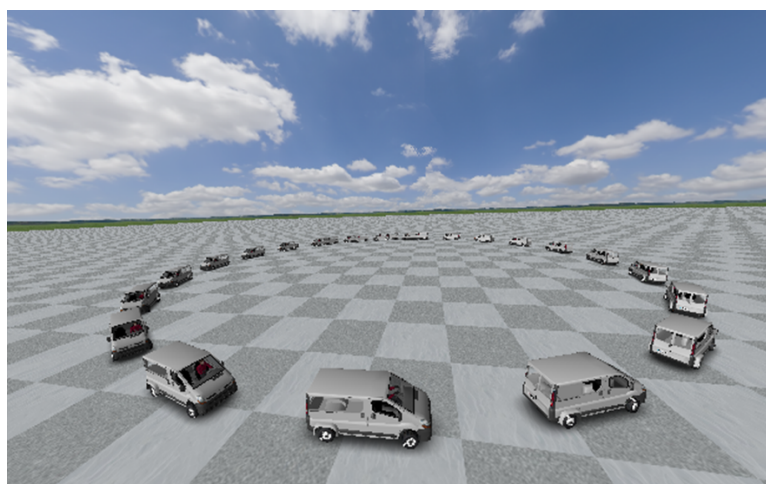
Figure 8. Simulated scenario for a Left J-turn maneuver in Trucksim®.
