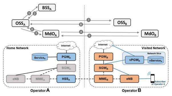
Figure 4-6. Workflow for virtualized roaming service creation
