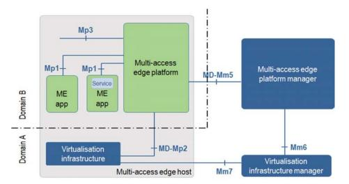
Figure 3-10. Integration at platform level with infrastructure owned by Domain A
