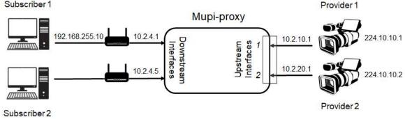
Figure 4-14. Experimental setup for the proof of concept
