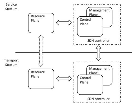
Figure 3-1. Cooperating Layered Architecture for SDN (CLAS)
