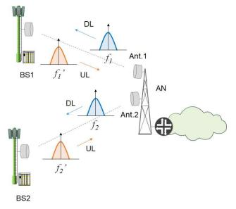
Figure 5-2. Low spectral efficiency case
