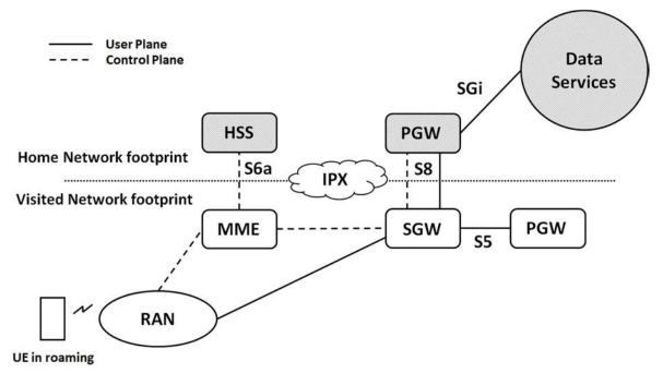
Figure 4-2. LTE roaming architecture (shadowed boxes represent home network elements)
