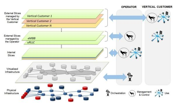
*Figure 2-4. Types of network slices according to management and control levels of responsibility*
