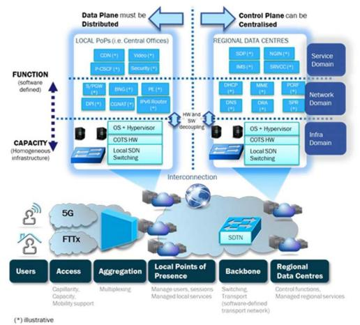
Figure 2-3. End-to-end virtualization [O10]
