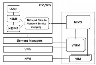
Figure 3-6. Mapping of the 3GPP network slicing concept to the ETSI MANO framework
