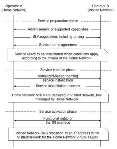
*Figure 4-5. Service preparation, creation and activation phases for the virtualized-based roaming service*
