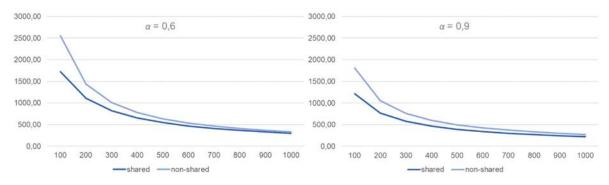
Figure 3-24. Variation on the number of total cached contents when increasing of vCache locations for 3000 selectable contents for 350000 simultaneous end users
