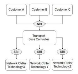
Figure 5-13. Transport Slice Controller concept
