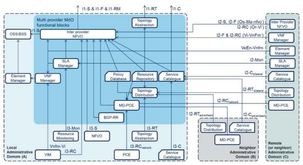
Figure 3-15. Functional model of multi domain orchestration
