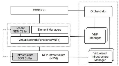
Figure 3-2. Applicability of CLAS in ETSI NFV environments [O24]
