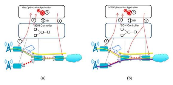
Figure 5-1. Selective traffic shaping (a) and re-routing (b)
