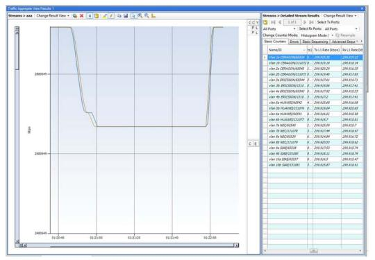
Figure 5-11. Capacity recovery after removing attenuation in the radio signal
