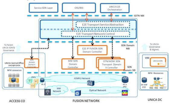
Figure 5-12. Telefonica's iFUSION architecture [A30]
