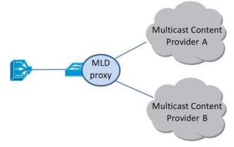
Figure 4-12. MLD proxy with multiple upstream interfaces
