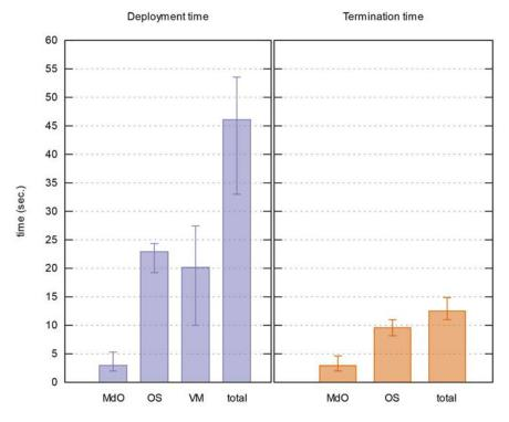
*Figure 4-9. Virtualized roaming service deployment and termination time (in total and per involved components)* [A14]
