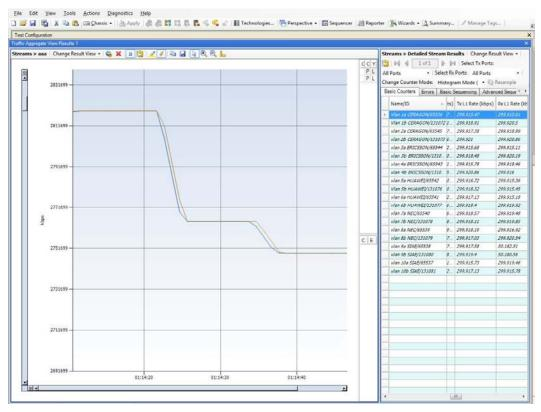
Figure 5-9. Capacity going below threshold after applying attenuation in the radio signal
