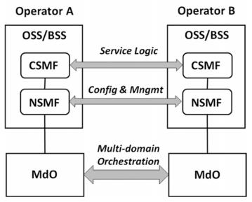
Figure 3-7. Complementary functionality for virtualized roaming service creation
