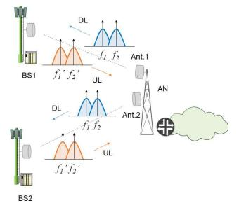
Figure 5-3. Full frequency reuse due to enough antenna separation
