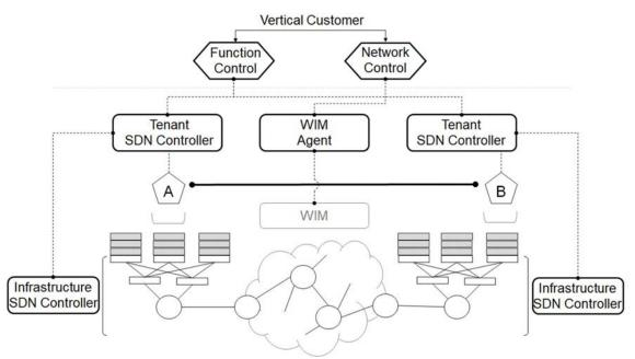
*Figure 3-3. Architecture enabling vertical customer control of service functions and their connectivity*
