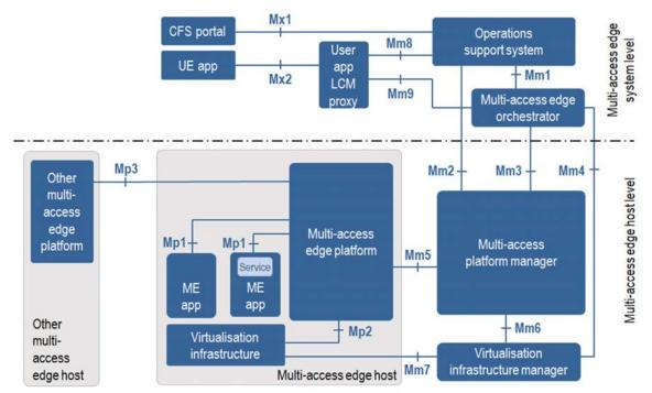
number of multi-access edge hosts and the multi-access edge management entities necessary to execute multi-access edge applications within an operator network.
