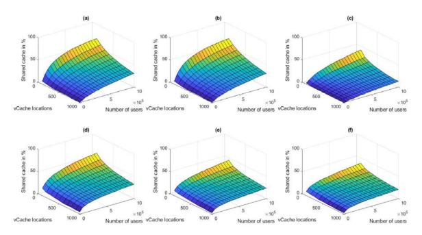
Figure 3-22. Efficiency E (in percentage) in terms of the average contents cached per location considering 100 to 1000 vCaches, and 10000 to 1000000 users uniformly distributed among the vCaches. Graphs show the results when α = 0,6 for 1000 (a), 3000 (b) and 5000 (c) contents, and similarly when α = 0,9 for 1000 (d), 3000 (e) and 5000 (f) contents
