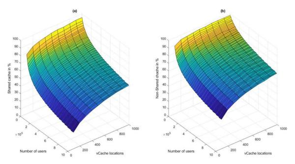
Figure 3-21. Percentage of the total number of cached contents in shared (a) vs non shared (b) approaches with respect to the number of end users (10000 to 1000000), for  $\alpha = 0.9$  and 3000 selectable contents as a function of the number of vCache locations (100 to 1000)
