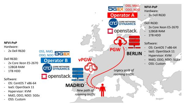
Figure 4-7. Experimental roaming setup consisting of two test-sites: Madrid and Berlin
