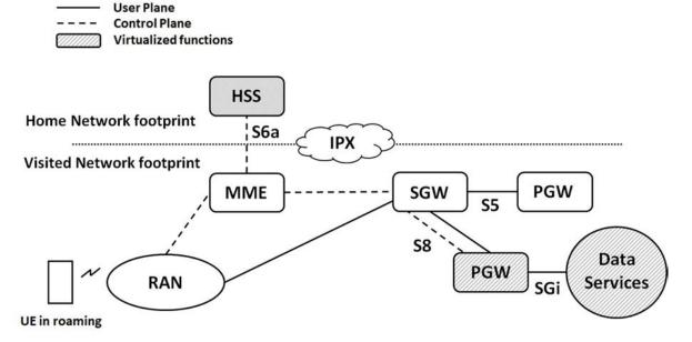
Figure 4-4. Virtualized-based LTE roaming architecture proposal (shadowed boxes represent home network elements, being virtualized the stripped ones)
