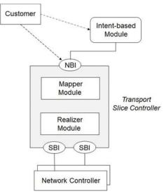
Figure 5-14. Proposed modular structure for TSC
