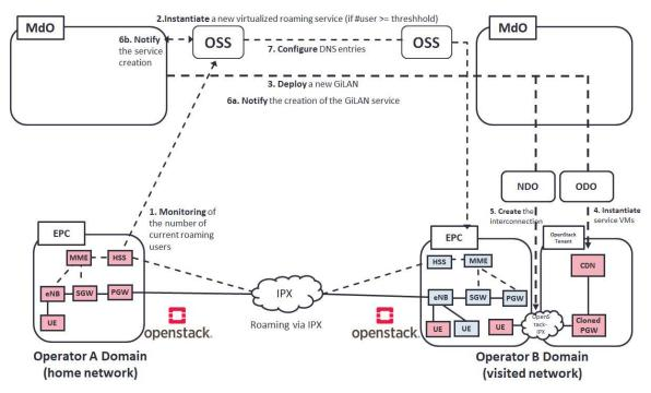
Figure 4-8. Experiment setup of the virtualized roaming service
