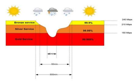
Figure 5-5. Example of capacity availability on the radio link due to weather conditions, reflecting the impact on link capacity and availability
