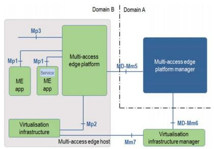
Figure 3-11. Integration at platform level with infrastructure owned by Domain B
