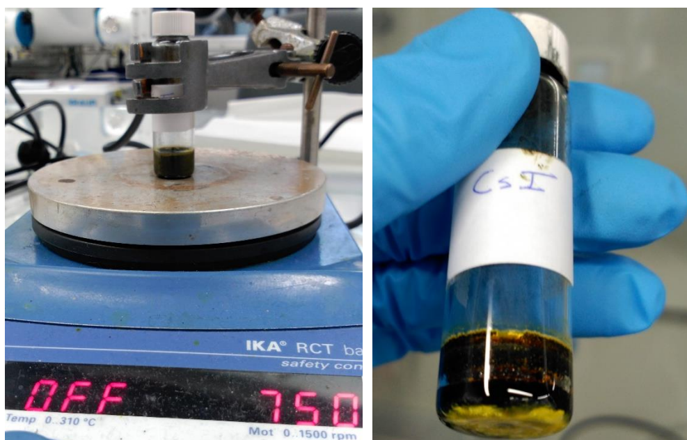
Figure 2-19 Black solution (left) containing 1mmol of CsI and 1mmol of SnI_2 in 1mL of acetone. Same vial after acetone evaporation (right).
