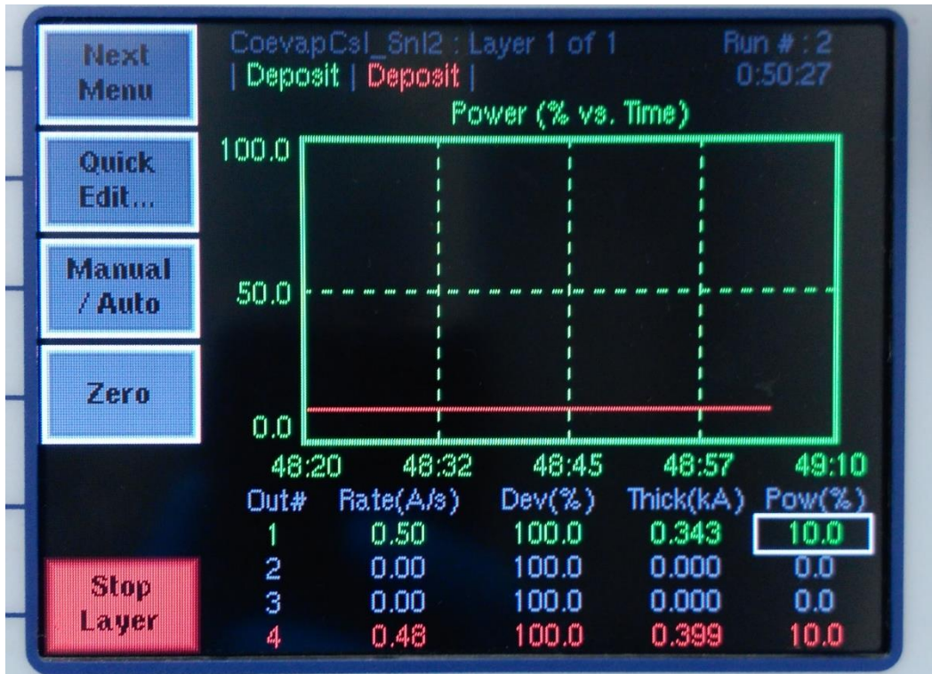
Figure 2-16 Deposition co-evaporation controller showing almost 1:1 deposition rates of CsI and SnI 2 .
