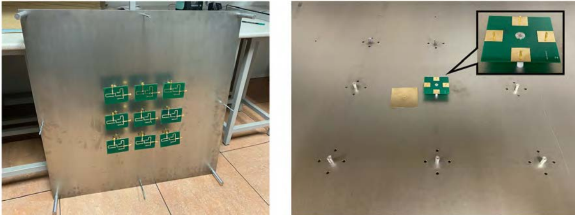
Fig. 4.26. On the left: the back side of the ground plane of the array, where the microwave circuits are located. On the right: the central element is shown with the top patch removed (shown at its side) for the feeding patches to be revealed. The locations where the other elements of the array will be placed, are also visible, with the central metallic ring.
