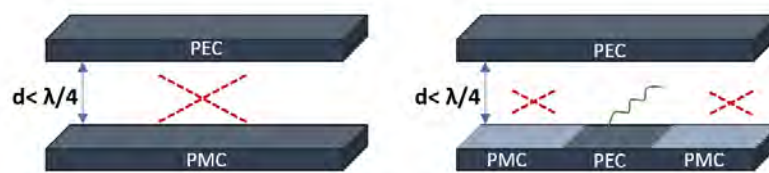
Fig. 5.1. The fundamental concept of gap waveguide technology. No modes can propagate between a PEC and a PMC for d < \lambda/4 (left). When we introduce a PEC zone in the PMC, propagation is supported (right).
