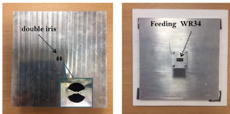
Fig. 2.19. A double iris slot was used as a radiation source (left). A standard waveguide transition was used to feed the iris slot (right).
