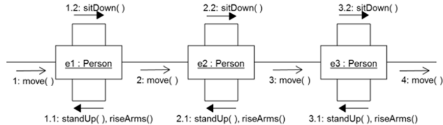
Figure 7: Wave Dynamics given by the UML Objects Diagram. One sees three instances of the Person, a Spectator in the crowd. The messages displayed for each person are: standup() and raiseArms(), sitDown() and finally move() to the next person.
