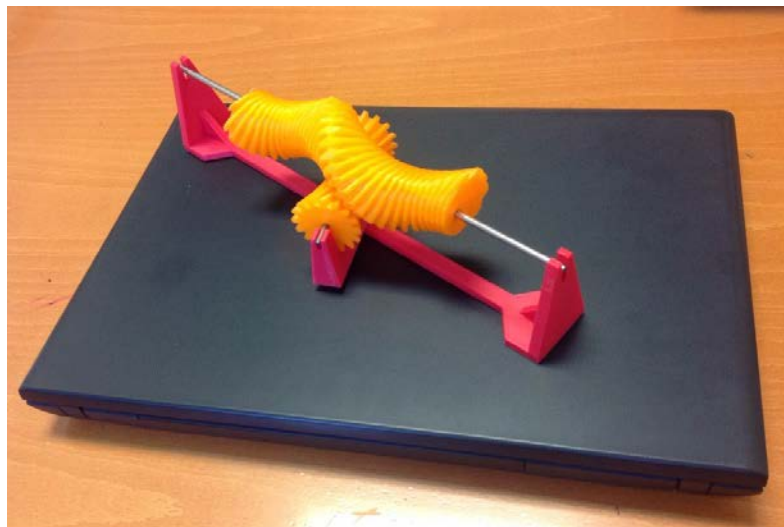
Fig. 11. The gear assembly produced on a 3D printer.
