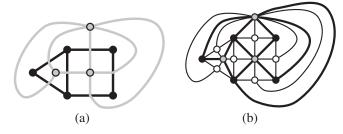
FIG. 1. (a) A dual pair G (black dots and lines) and  $G^*$  (gray dots and lines). (b) The quadrangulation  $\hat{G}$  (black or gray dots and thick lines) and triangulation  $\tilde{G}$  (all dots and lines).
