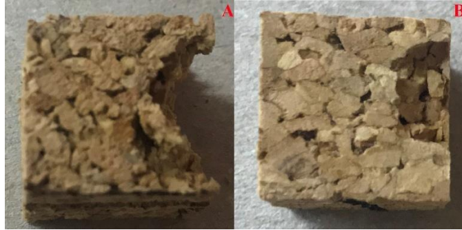
Figure 95: Damage mode of NL10 (A) and NL20 (B) specimens tested at 7 J and -40 °C
