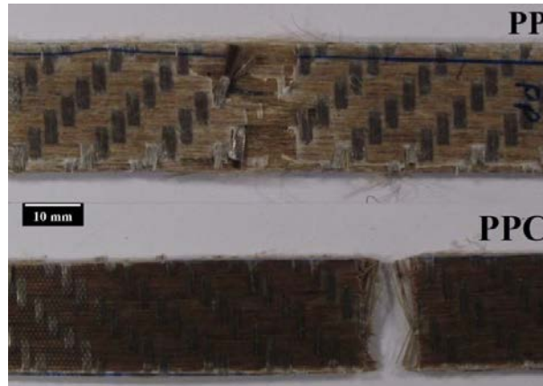
Figure 154: PP and PPC samples damage mode along basalt and flax direction, respectively
