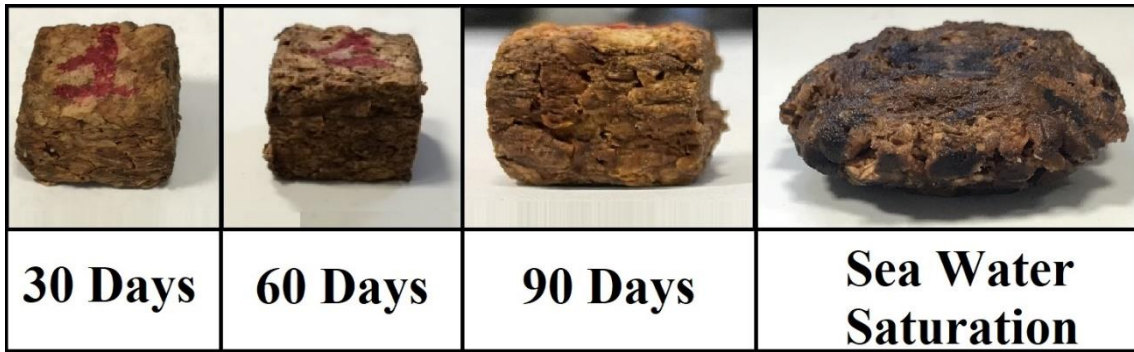
Figure 82: NL25 samples deformation mode as a function of salt fog and sea water exposure time
