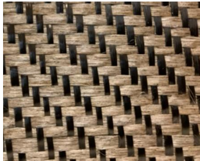
Figure 11: LINCORE® HF T2 360 flax/basalt hybrid twill woven fabric employed as skin reinforcement
