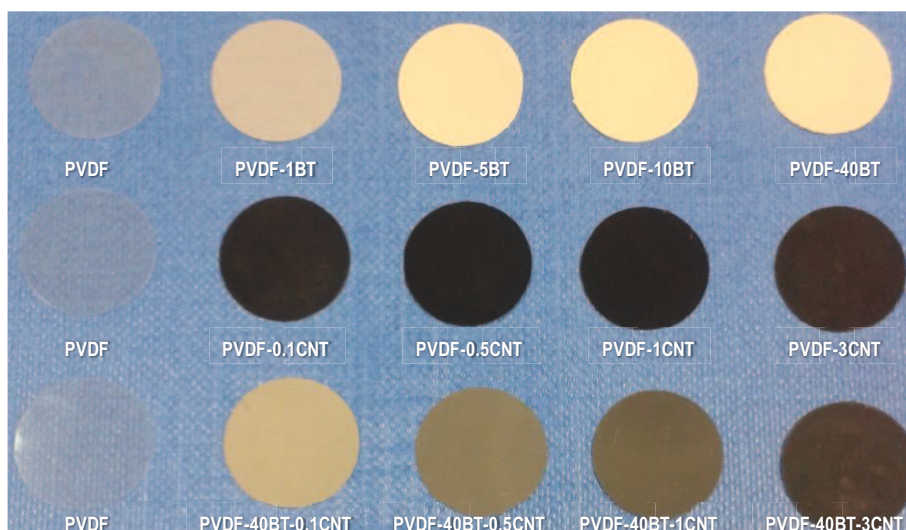
Figure 1. Specimens prepared form films of PVDF containing BaTiO 3 and MWCNT (see Table 1 for nomenclature).
