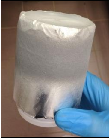
Fig. 1 Mat of PVDF/MWCNT material deposited on a cylindrical collector.
