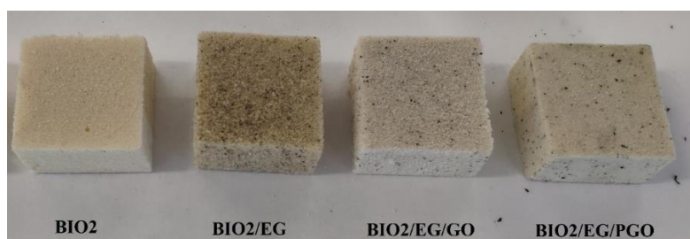
Figure 7-7. Physical structure of the different foam samples studied.
