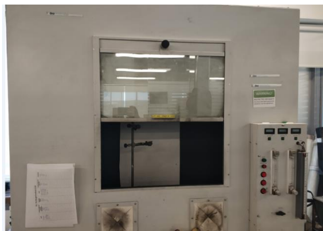
Figure 3-1. Picture of the vertical burning test (UL94) chamber.
