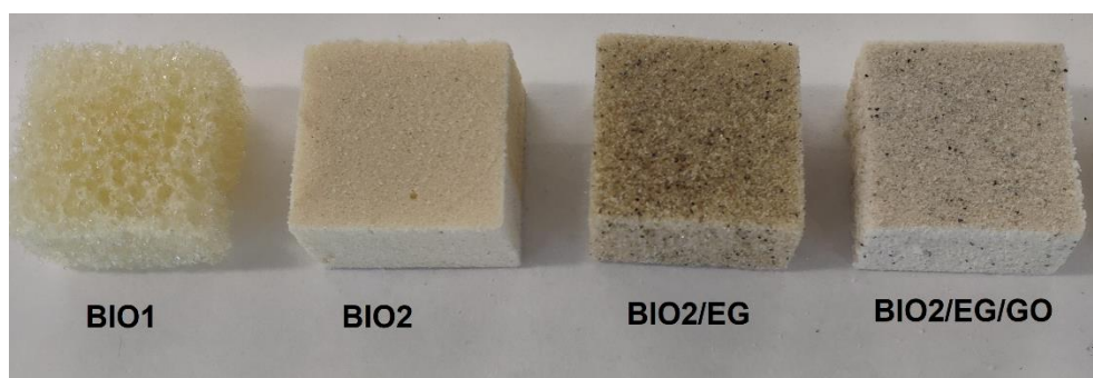
Figure 6-9. The different studied biobased-RPUF samples showing their different physical structure.
