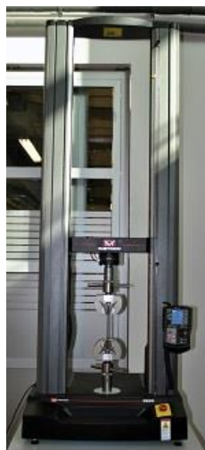
Figure 3-2. Picture of the dual column tabletop universal testing system (INSTRON 5966).
