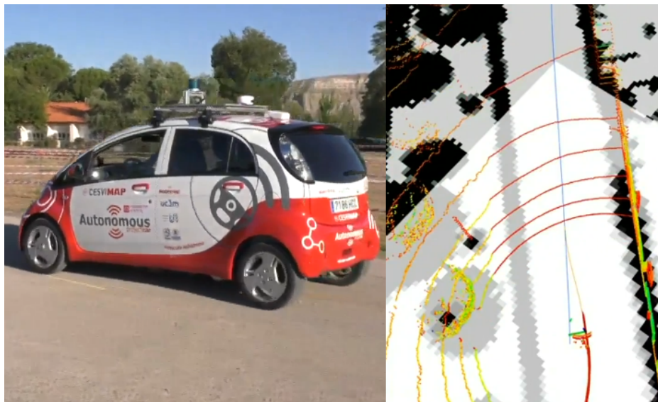
Figure 6. Our autonomous vehicle platform testing the proposed method (left), and a visualization of the LiDAR pointcloud and the map (right).
