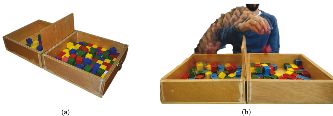
Figure 1. The classical Box and Blocks Tests (BBT): (a) components: wooden box and colored cubes; (b) mechanics: user performing the test.
