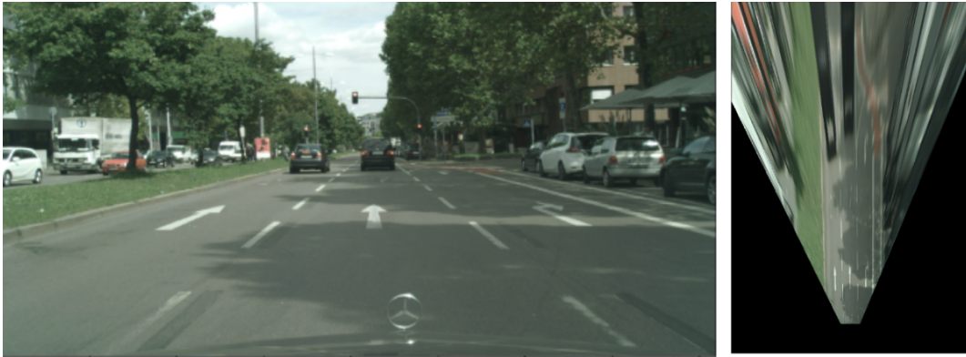
Figure 2.4: Transforming an image into bird's eye view using IPM [24].
