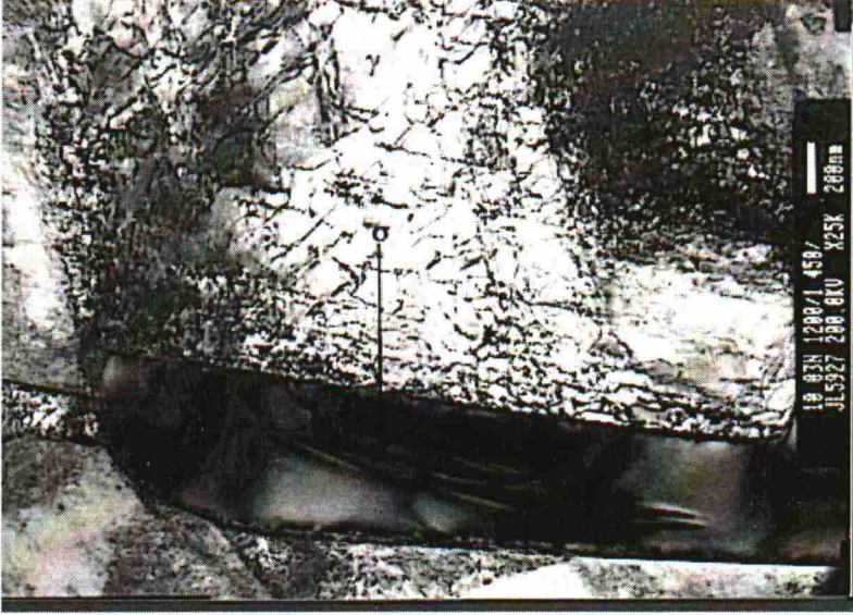
Figure 29. Intergranular \sigma phase in SMO 0,3N isothermally annealed at 450 °C for 500 h.
