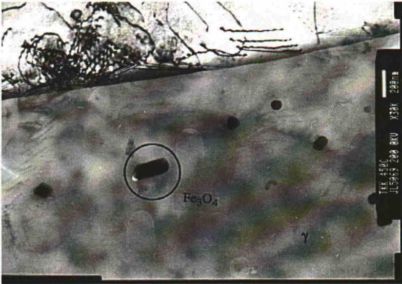
Figure 30. Fe-oxides of type \text{Fe}_3\text{O}_4 in SMO 0,5N1 isothermally annealed at 450 °C for 1 h.
