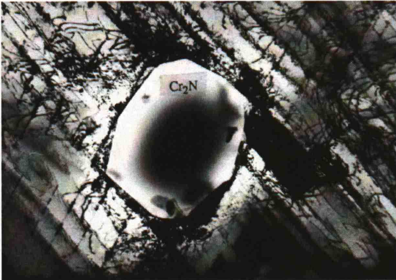
Figure 26. Intragranular \text{Cr}_2\text{N} precipitate in SMO 1,15N. Magnification 18500 x.
