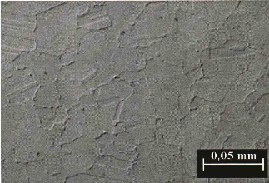
Figure 22. Microstructure of SMO 0,3N annealed for 500 h at 450 °C showing intergranular precipitation.
