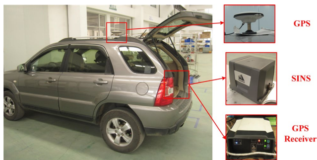
Fig. 8. Practical test vehicle platform.
