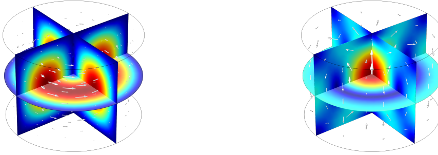
Figure 2.5: Left: Electric field norm of a cylindrical cavity \text{TE}_{011} mode. Right: Magnetic field norm of a cylindrical cavity \text{TE}_{011} mode. Arrows show field direction and have size proportional to strength, while the heat map shows relative magnitude of the norm.
