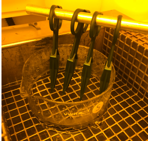
Figure F.1: Four chip pieces (to create two full chips), suspended on Nalgene forceps into a beaker of 1165 remover, which is itself in a heated bath with sonication. This method was used also for cleaning individual chips with IPA and DI.
