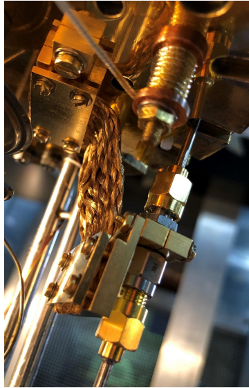
Figure 3.4: Figure showing the floating braid thermalisation for attenuators.
