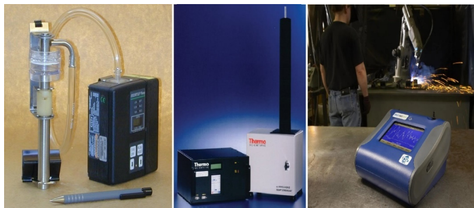
Figure 1. Devices used in PM measurement campaigns conducted within the Parisian underground subway: Left: Gravimetric method equipment [41]; Middle: TEOM (model: 1400; brand: Thermo Scientific); Right: DustTrack (model: DRX; brand: TSI).
