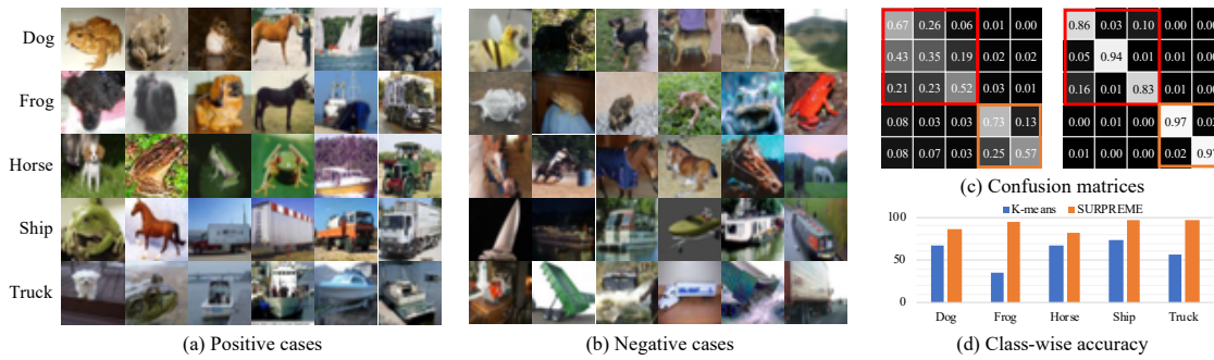
Figure 5.6: Qualitative studies on CIFAR-10. (a) Samples that were wrongly classified by k-means but corrected by SUPREME. (b) Samples that were wrongly classified by SUPREME. (c) Confusion matrices yielded by k-means (left) or SUPREME (right). (d) The clustering accuracy of k-means or SUPREME on each target category.
