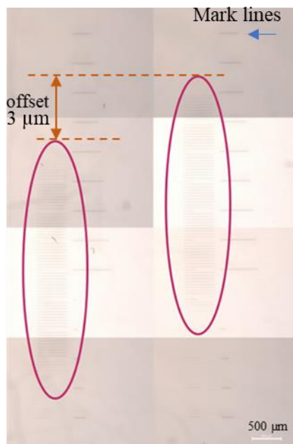
Figure 3.6 Two sets with the same pulse energy: 0.18 \mu\text{J} , and marks beside the sets. The ellipses highlight areas where the lines are visible.
