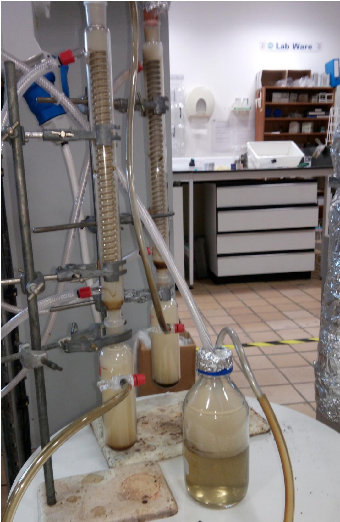
Figure 7-4: Appearance of gas as it enters the condensation train and gas scrubbing
