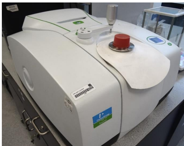
Figure 3-8: PerkinElmer Frontier FTIR analyser used during analysis
