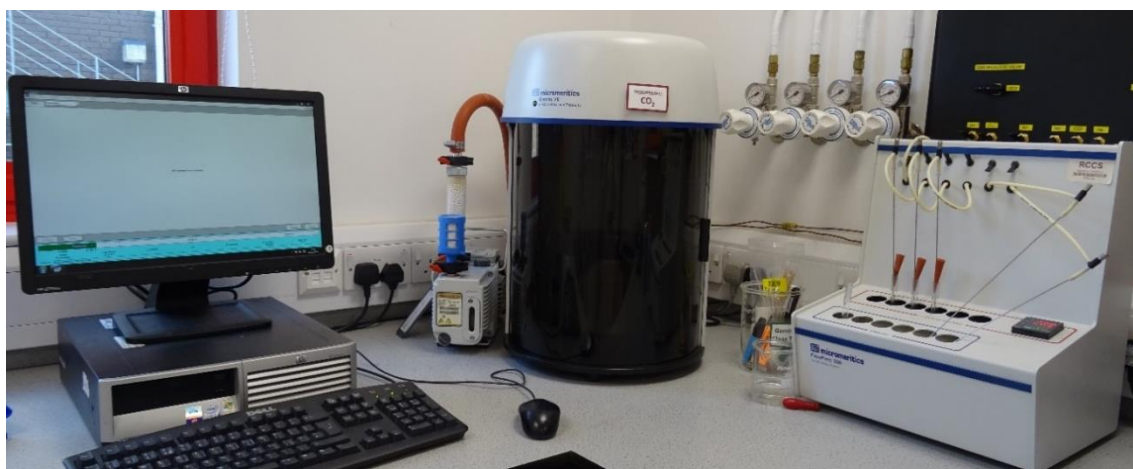
Figure 3-11: Micrometric Gemini VII and degassing heater configuration
