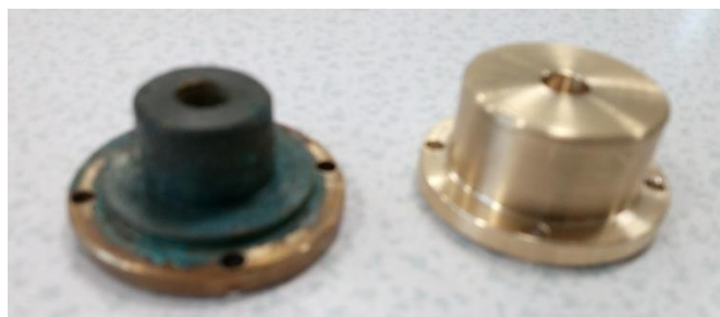
Figure 4-20 Old bearing (left) Vs. the re-designed bearing (right)
