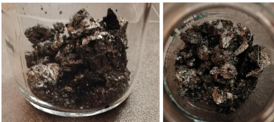
Figure 7-1: Char appearance in the auger feeder
