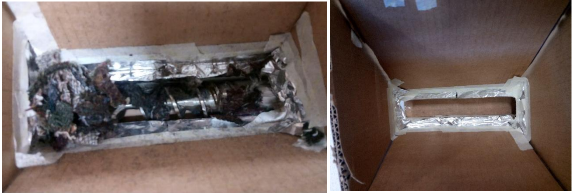
Figure 4-18: The prototype made for setting the angle of the hopper (right hand side with no auger and deed, left with auger and wool in the hopper)
