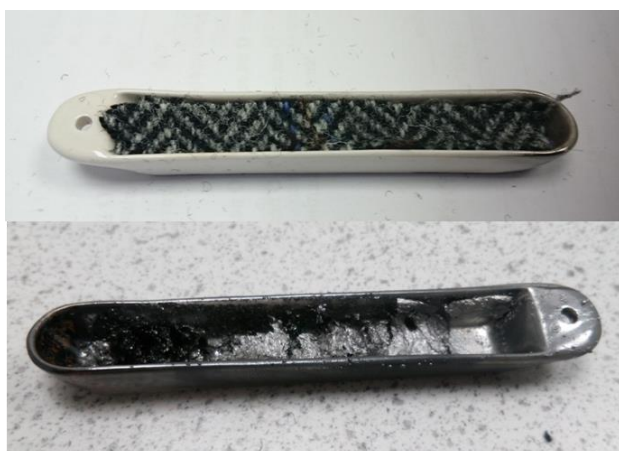
Figure 6-4: Wool before pyrolysis (top), After pyrolysis in the ceramic boat (bottom)
