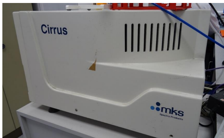
Figure 3-10: MKS Cirrus MS analyser used for gas analysis
