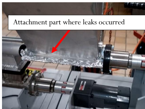
Figure 4-25: The attachment point of the new hopper to the tubing 1 where leaks occurred; fire cement was used with additional aluminium tape on top of it
