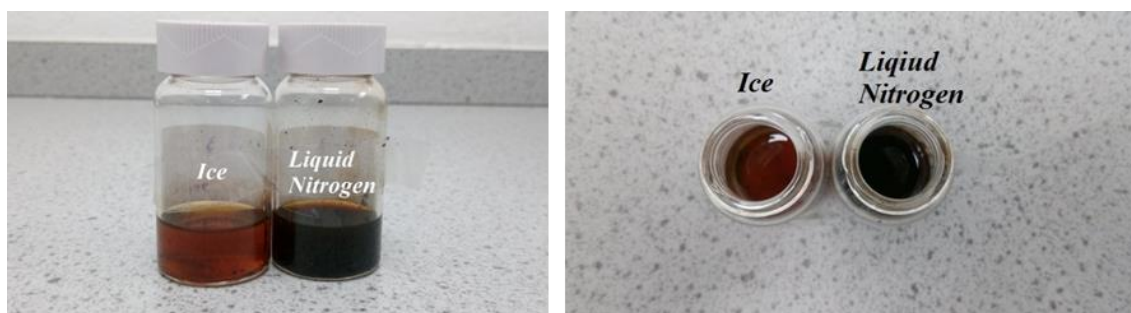
Figure 6-11: Comparison between the appearance of the oil products obtained from pyrolysis at 800 Celcius
