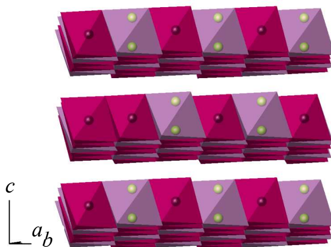
Figure 57: The two-layer structure of \text{Cr}_{0.5}\text{In}_{0.5}\text{GeTe}_3 .
