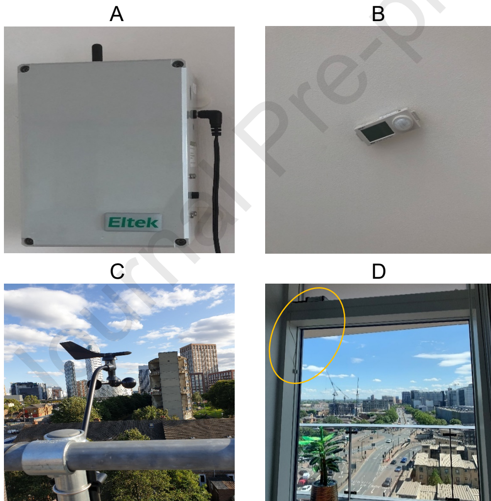
4 Figure 2. Photos of equipment. A: Eltek IAQ 110; B: HOB0 UX90; C: Davis 6410; D: 5 Eltek GS34.
