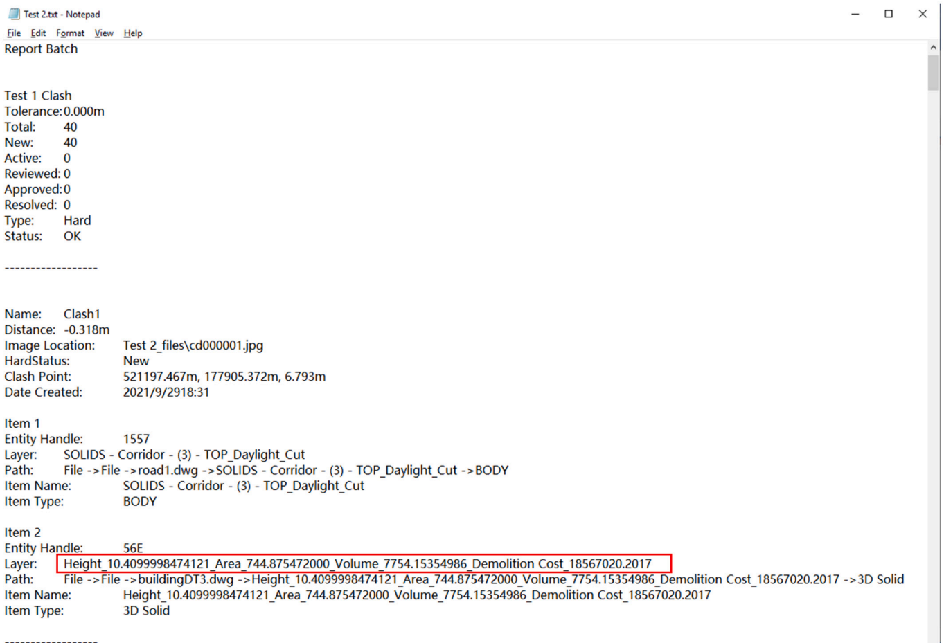
Fig. 24. Clash detection report and BIM models' information for building demolition costs estimation.
