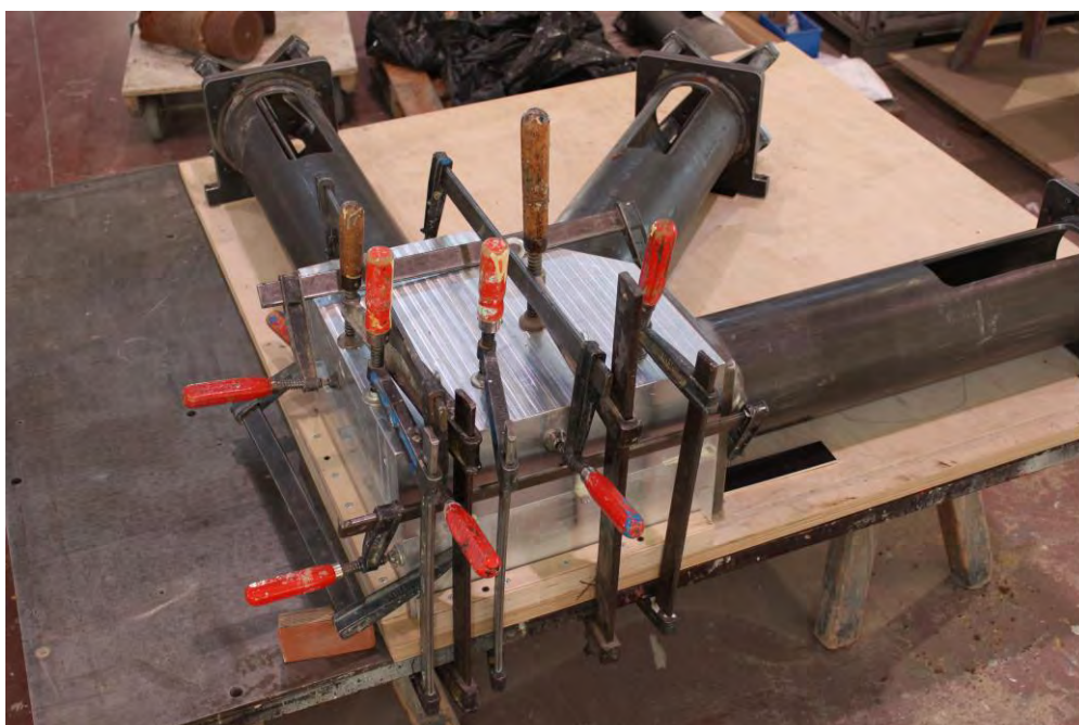
Fig. 5-45 Vacuum pressed fabrication of WFC joints (Prototype)
