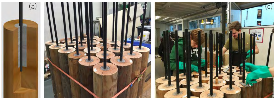
Fig. 4-1 Modified bonded-in threaded rods: longitudinal section sketch (a), cross-section view (b) and fabrication of test specimens (c)
