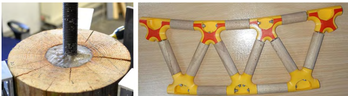
Fig. 1-2 Modified bonded-in rods (left) and model of moulded joining technology (right)
