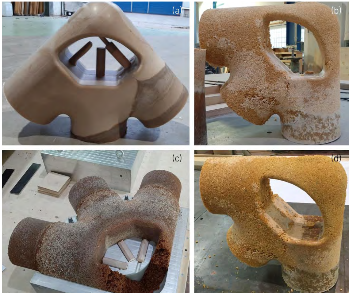
Fig. 5-46 Evolution of joint prototype fabrication composed of PC (a) and WFR (b-d)
