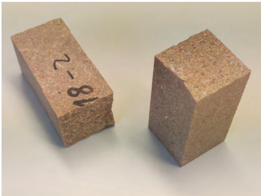
Fig. 5-39 Fracture surface of wood-fibre composite in flexural tests
