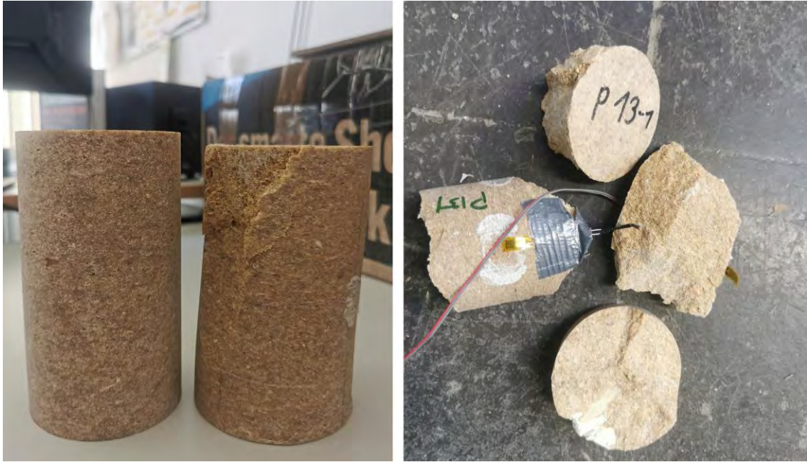
Fig. 5-37 Ductile (left) and sudden brittle (right) failure of cylindrical WFC specimens
