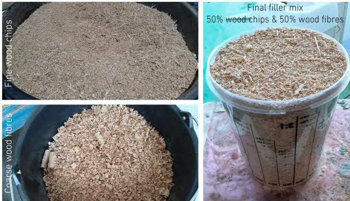
Fig. 5-32 Filler mix for wood-fibre resin test specimens
