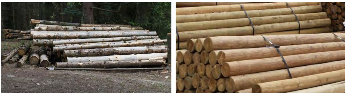
Fig. 1-1 Logs (left) and structural roundwood (right)
