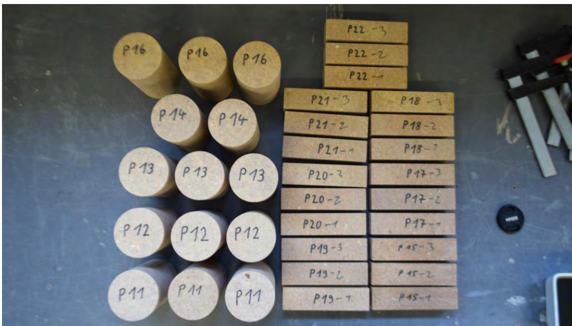
Fig. 5-34 Wood-fibre composite test specimens (production batches 1 - 12)
