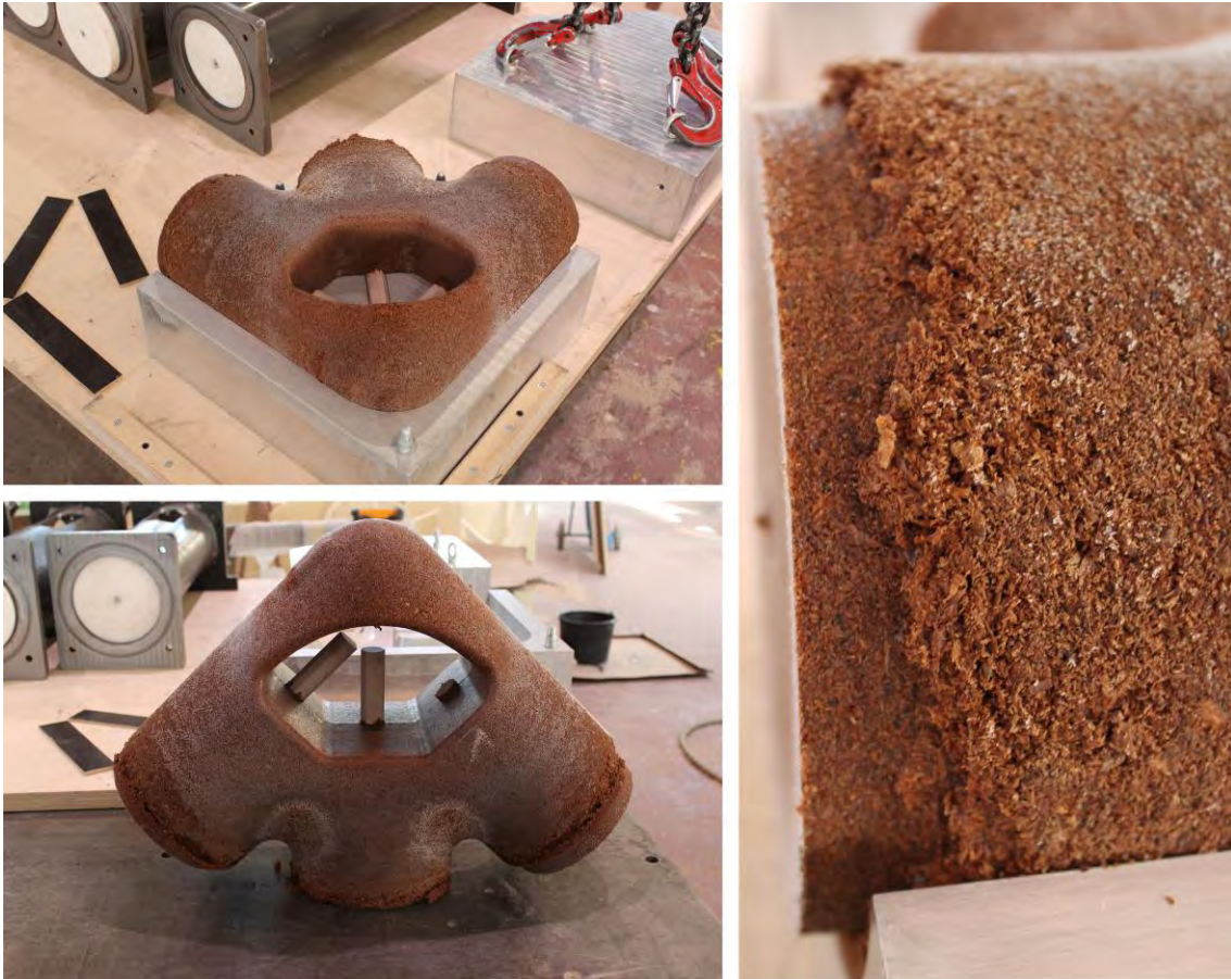
Fig. 5-47 Optimized joint prototype fabrication composed of WFR
