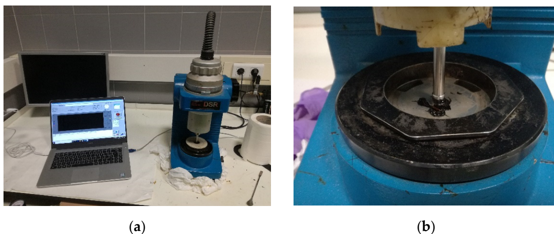
Figure 2. (a) Dynamic shear rheometer; (b) Testing sample on 8 mm geometry.
