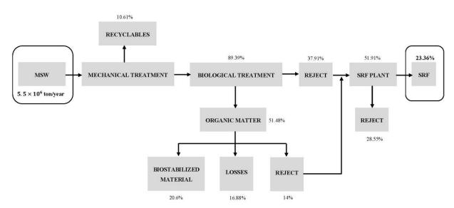
**Figure 4.** Flowchart of the process showing the mass balance (in % of the initial  $5.5 \times 10^6$  ton/year) [68].
