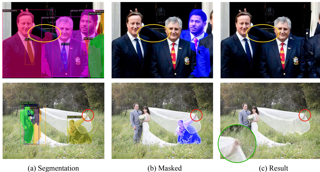
Fig. 5.16: Failure cases due to the failed segmentation. The failures in segmentation will generate incorrect masks, affecting the final inpainting results.
