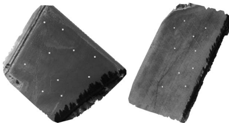
Figure 3. Orthomosaic pictures from the NIR spectral band. In the images, the multiple white squares are the ten measurement points of the crop properties. The image of the Mölylä field (left) was taken on 31 July 2019 at 12:00 and the image of the Koirasuo field (right) on 1 August 2020 at 12:00.
