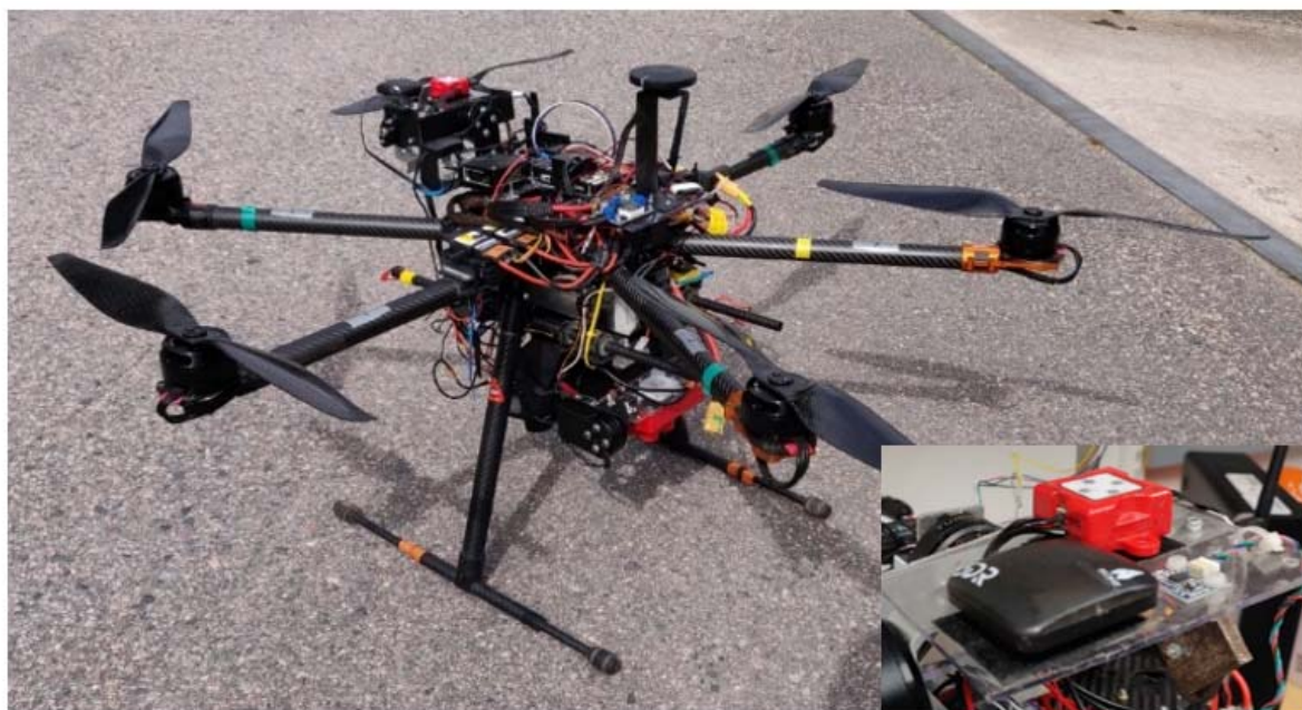
Figure 1. Custom-built drone with a Tarot T960 frame. The multispectral camera light sensor had a separate gimbal (small figure). This solution minimizes disturbances that are caused by shadows forming on the sensor when the drone is flying away from the sun.
