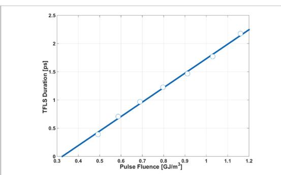
**Figure 2.** Relationship between the fluence of laser pulse and the duration of TFLS. The circles represent the duration of TFLS under different fluence, and the line is fitted to illustrate the evolution of duration of TFLS.
