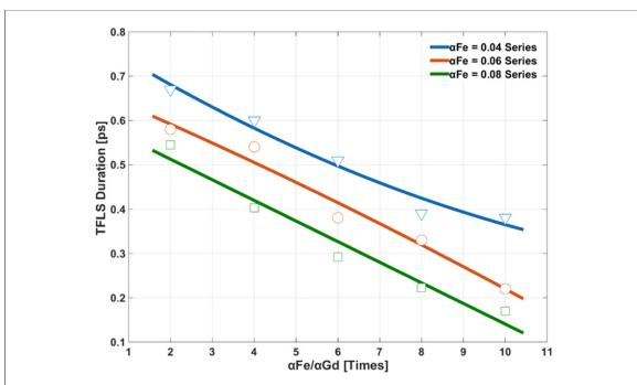
**Figure 5.** Relationship between damping and the duration of TFLS. The horizontal axis represents the ratio of Fe damping to Gd damping. Data points represent the duration of TFLS at different damping ratio. The colors of the lines represent different damping values.
