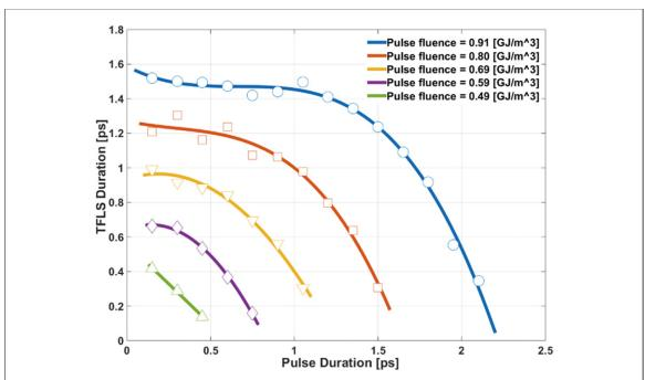
**Figure 4.** Relationship between the duration of laser pulse and the duration of TFLS. The data points represent the duration of TFLS under laser pulse with different duration. Data points represent the duration of TFLS at different pulse duration. Different colored lines represent different fluences of laser pulse.
