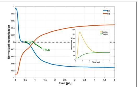
**Figure 1.** Diagram of laser-induced ultrafast magnetization dynamics. The blue line and red line represent the magnetization evolution of Fe and Gd, respectively. In the ellipse area, the magnetization of Fe and Gd are in the same direction, which represents TFLS. (Inset) Time dependence of the electron and phonon temperature from the two-temperature model. The yellow line and green line represent the temperature evolution of electron and phonon, respectively.
