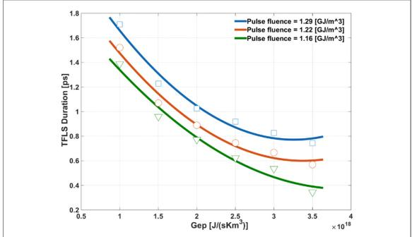
**Figure 6.** Relationship between electron phonon coupling coefficient  $G_{ep}$  and TFLS. Data points represent the duration of TFLS with different  $G_{ep}$ . Different colored lines represent laser pulse with different fluences.
