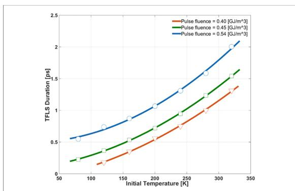
**Figure 3.** Relationship between initial temperature and TFLS. Data points represent the duration of TFLS at different initial temperatures. Data points represent the duration of TFLS at different initial temperature. Different colored lines represent different fluences of laser pulse.
