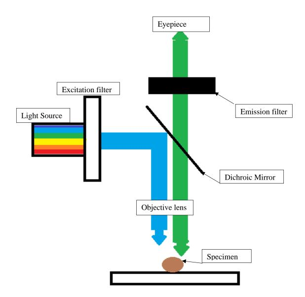
Figure 9 Schematic demonstration of a fluorescent microscope. The excitation filter permits only the desired wavelength of light to pass through. The light is reflected off the dichroic mirror to illuminate the fluorophore bound to the specimen. Emitted light from the fluorophore passes through the dichroic mirror and emission filter to the eyepiece.
