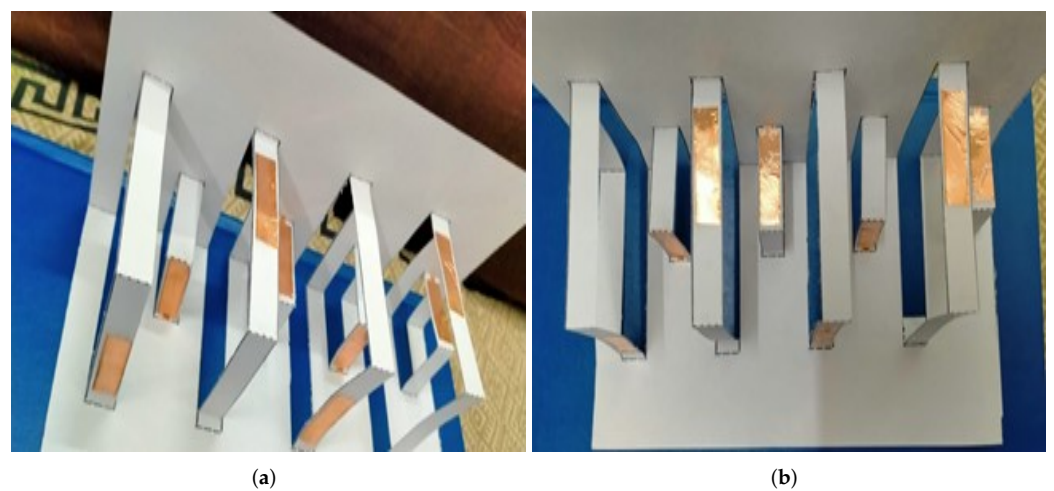
Figure 3. Kirigami MIMO antenna: (a) perspective view; (b) front view.
