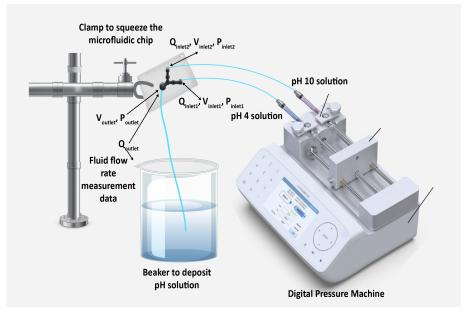
**Figure 2.** Using digital pressure machine, experimental measurement set up of a PDMS-made microfluidic chip to determine data of microfluidic parameters.
