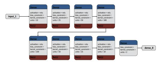
**Figure 4.** The algorithm of the internal architecture of the dense layers of the ReLU, leaky ReLU, and Swish basic functions applied to analyze the microfluidic parameter data.
