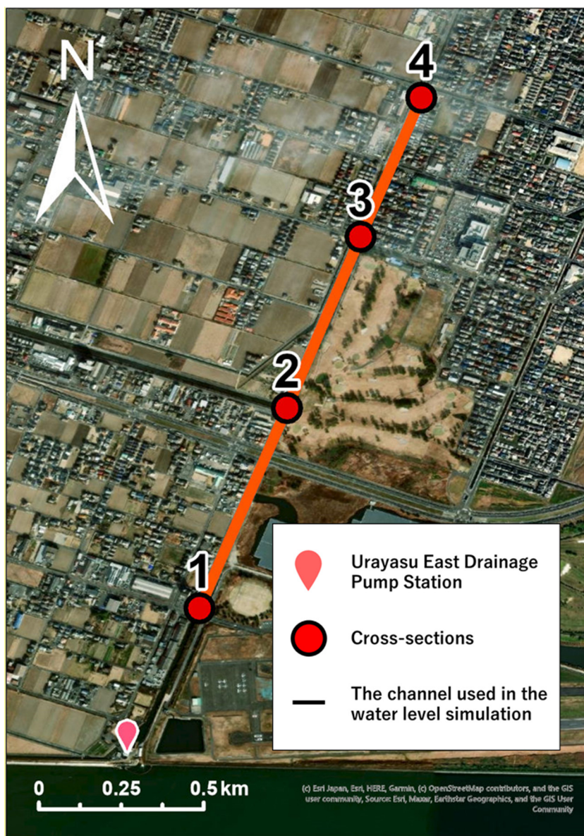
Figure 3. Urayasu East Drainage Pump Station channel map. Cross-sections were used when points to change parameters as the channel structure changes. Copyright: Esri Japan, Esri, HERE, Garmin; OpenStreetMap contributors, and the GIS user community. Source: Esri, Maxar, Earthstar Geographics, and the GIS user community.
