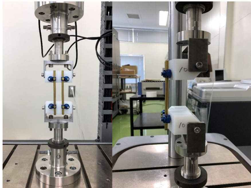
Figure 1. Test specimen installed on the Instron 8521.
