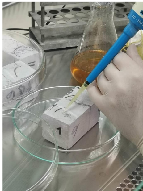
Figure 3. Application of bacteria-based repair agent onto an artificially generated crack on cement mortar beam (authors' image).
