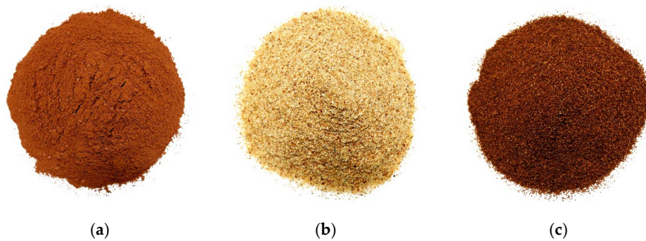
Figure 1. Photographs of raw materials: (a) red clay; (b) sawdust; (c) coconut coir dust.
