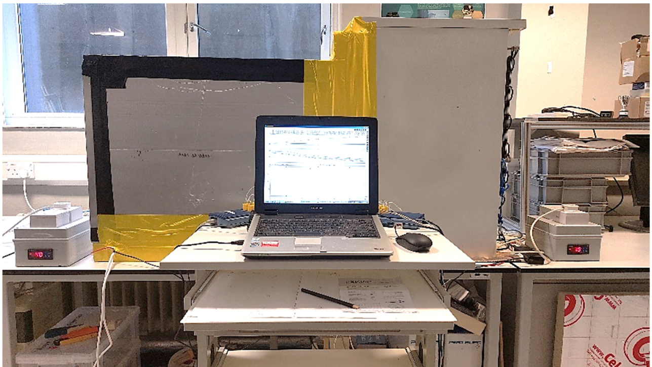
Figure 6. Test setup of thermal transmittance measurement.
